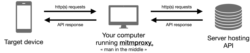
Figure 2.2: The simple architecture of a Man-in-the-Middle (MITM) interception using mitmproxy.
